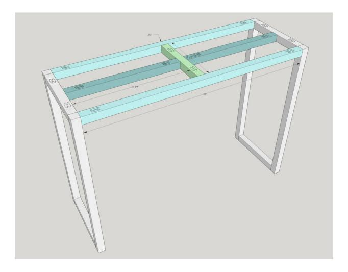
Construct the carcass. Drill 1  $\frac{1}{2}$ " pocket holes into the 45" rails and attach to the legs with 2  $\frac{1}{2}$ " pocket hole screws. Find the midpoint and attach the middle 2x2 board with 2  $\frac{1}{2}$ " pocket hole screws and wood glue. Add the 21  $\frac{3}{4}$ " pieces in the same way.
